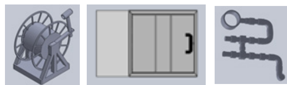
Figure 10. Designs of parts for the unit of coiled tubing in SolidWorks (reel, toolbox, manifold) / Figura 10. Diseños en Solid Works de piezas para la unidad de coiled tubing (Rollo, caja de herramientas, manifold)
