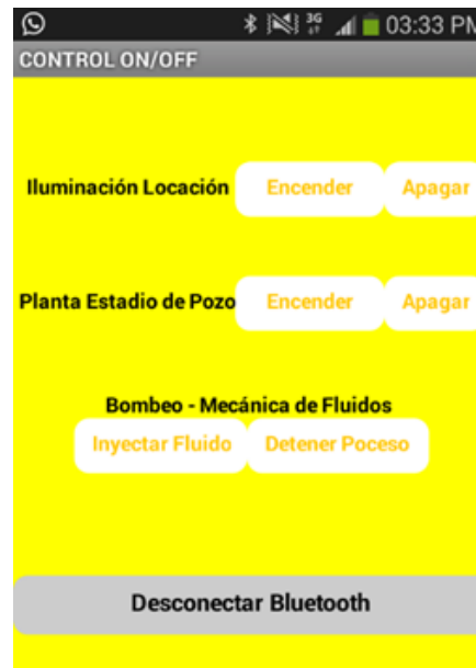
Figure 23. Screenshot of graphical interface of the ON/OFF control system of the Android mobile application / Figura 23. Screen interfaz gráfica del sistema de control ON/OFF de la aplicación móvil Android
