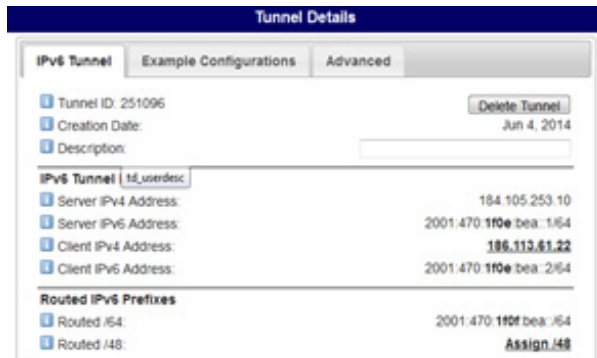
Figure 4. Tunnel details / Detalles del Túnel
