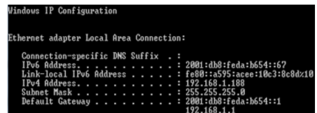
Figure 2. Dual stack feature in a Windows® client / Característica Dual Stack en cliente Windows
